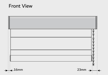
All component parts and fabric are enclose within a rounded resulting in a compact, robust system with a streamlined appearance. Fast, multiple installations can be achieved using top fix or face fix brackets that can be fitted along the whole length of the cassette. The snap fix fascia can be white or graphite or with a matching fabric profile.
