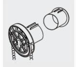
Side action control unit & plunger in engineered plastic. Unit locks into brackets. Clutch type suitable up to 9kg weight. Can be left or right control.
