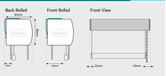
All component parts and fabric are enclose within a rounded resulting in a compact, robust system with a streamlined appearance. Fast, multiple installations can be achieved using top fix or face fix brackets that can be fitted along the whole length of the cassette. The sna fix fascia can be white or graphite or with a matching fabric profile.
