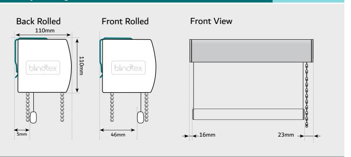
All component parts and fabric are enclose within a rounded resulting in a compact, robust system with a streamlined appearance. Fast, multiple installations can be achieved using top fix or face fix brackets that can befitted along the whole length of the cassette. The snap fix fascia can be white or graphite or with a matching fabric profile.
