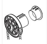
Side action control unit & plunger in engineered plastic. Unit locks into brackets. Clutch type suitable up to 9kg weight. Can be left or right control.
