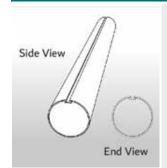
The design allows for full integration of the selected fabric and also provides maximum resistance to tube deflection.
